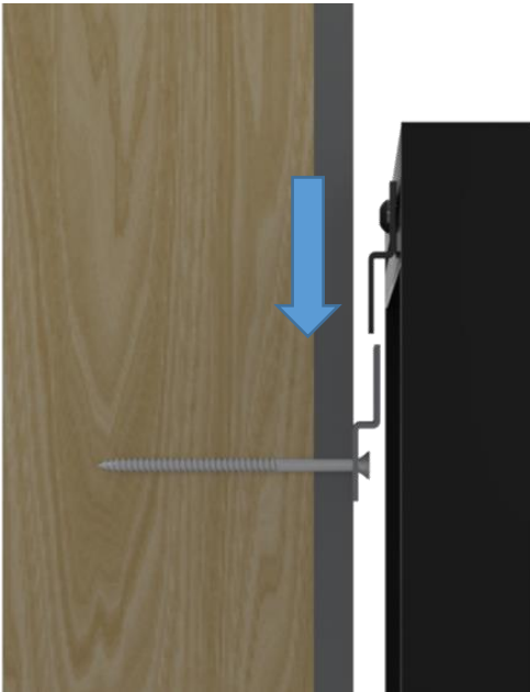
Figure 6: Side view render of WSDQ showing action needed to mount frame to wall mounted bracket.
